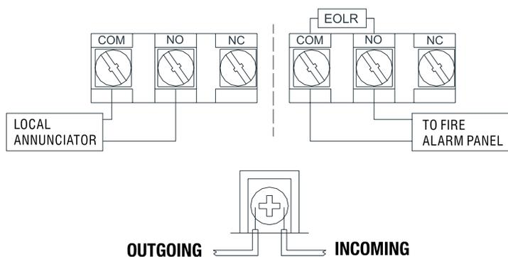
An uninsulated section of a single conductor should not be looped around the terminal and serve as two separate connections
